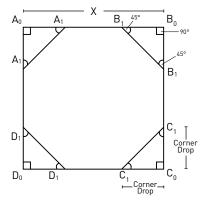
2. To find the corner drop (the distance from the corner of the square A0 to the octagon corner A1), multiply the length of side X by 0.2929.
