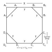
3. When staking out the eight corners of the octagon, multiply the length of side X by 0.4142 to verify that each side of the octagon is equally sized and the corners are properly located.
